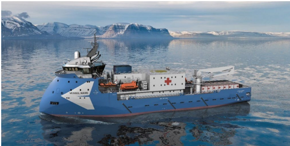
Figure 10. Lateral view of a permanent PSV conversion to Hospital and Aid Ship.
