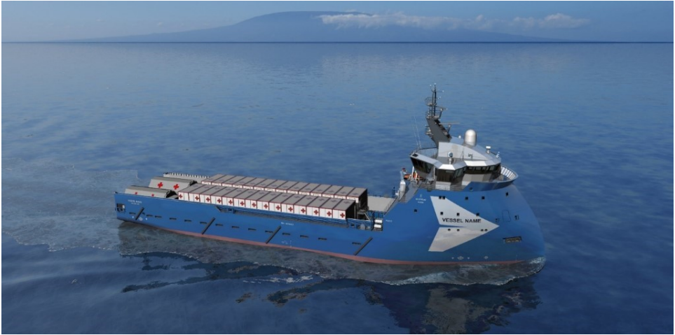
Figure 8. Lateral view of a temporal PSV conversion to Hospital and Aid Ship.
