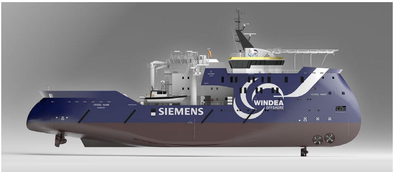
'Windea La Cour', the first vessel featuring an X-BOW® as well as the novel X-STERN™, was ordered by Bernhard Schulte Ship-management, and delivered in 2016. The sister vessel, 'Windea Leibniz', delivered one year later, is X-BOW® vessel number 100.
