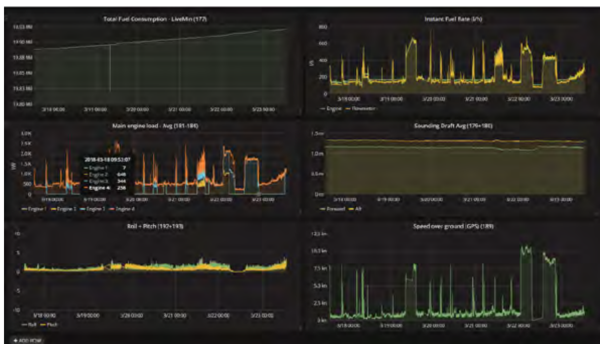
Figure 2: Example of dashboard made in Grafana to present data from Blue Box™.
