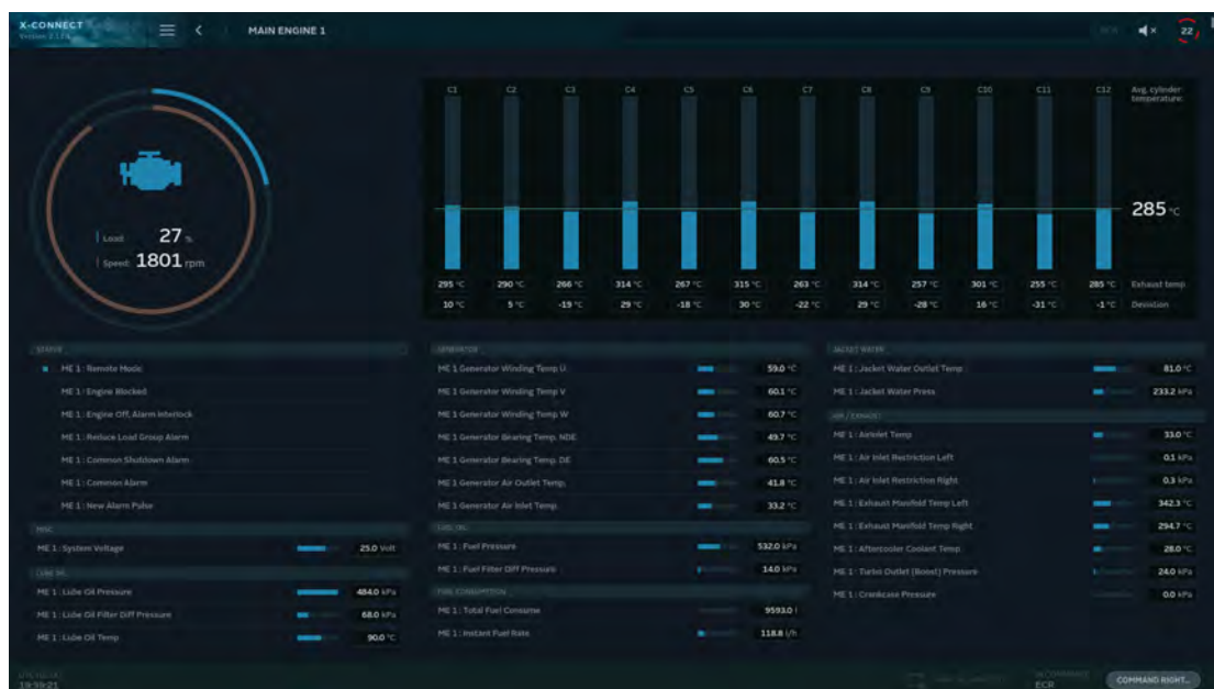
Figure 16: Main engine view - engine cylinder animation, bar graph representation of signal list
