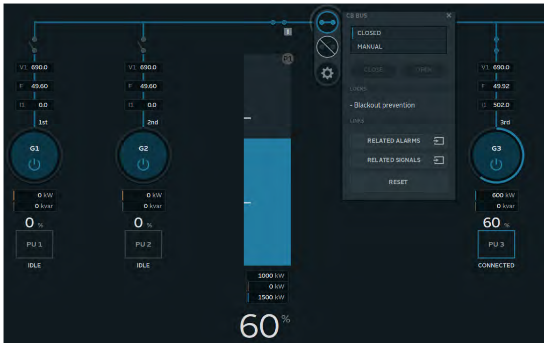
Figure 7: Circuit breaker is blocked from opening to prevent blackout
